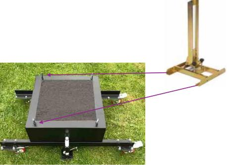
Once the concrete has dried, attach the bolt down mast base to the top ond bolt down with the four nuts supplied.
