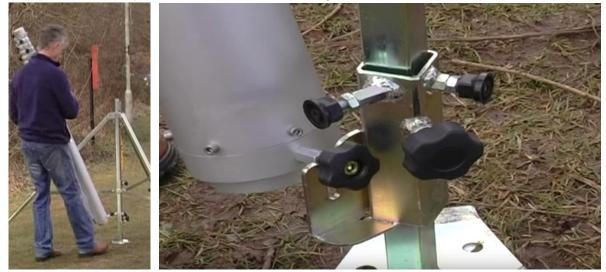
Offer the thumbscrew at the lower end of the mast to the bottom Q-Pod slot, without lowering it fully into the slot...
