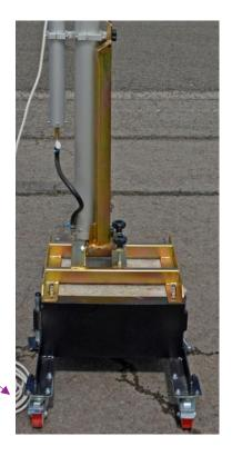
Lower the two support plates to the ground for extra stability.
