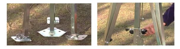
Stand Q-pod upright and turn the centre knob to locate centre pole as required
