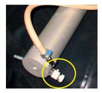
The presence of other residue (apart from water) might indicate internal damage to the mast.
