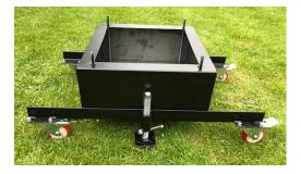
The shell must be filled with concrete before first use. The concrete is a mixture of cement, sand (aggregate) and water.
