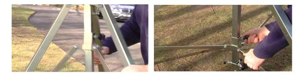
Pull down the centre column to open out the legs, and secure as shown
