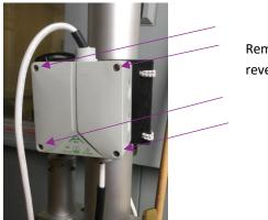
Remove screws to reveal dimmer toggle
