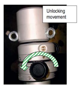
5. Extend fully the first section using the hand pump. When fully extended lock the section by turning knob clockwise and proceed with the second section (next one down from top) by unlocking it, pumping, locking and so on until the desired height is reached or to complete extension of the mast.
