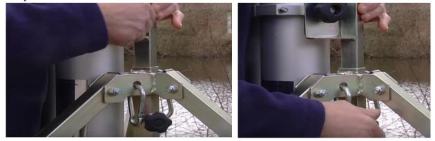
Locate the top slot and align the top thrumbscrew on the mast to the top slot on the Q-Pod and drop it into place. Tighten up both thumbscrews to secure. A large washer should be positioned behind each thumbscrew.
